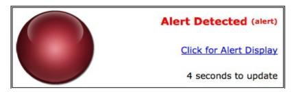
Clicking on the displayed link ("Click for Alert Display"), will bring up the "View Alerts" page in the main browser window showing the device which caused the alert to trigger. The "View Alerts" page will then also allow displaying map for the selected device causing the alert, or clearing the alert once it has been handled.
